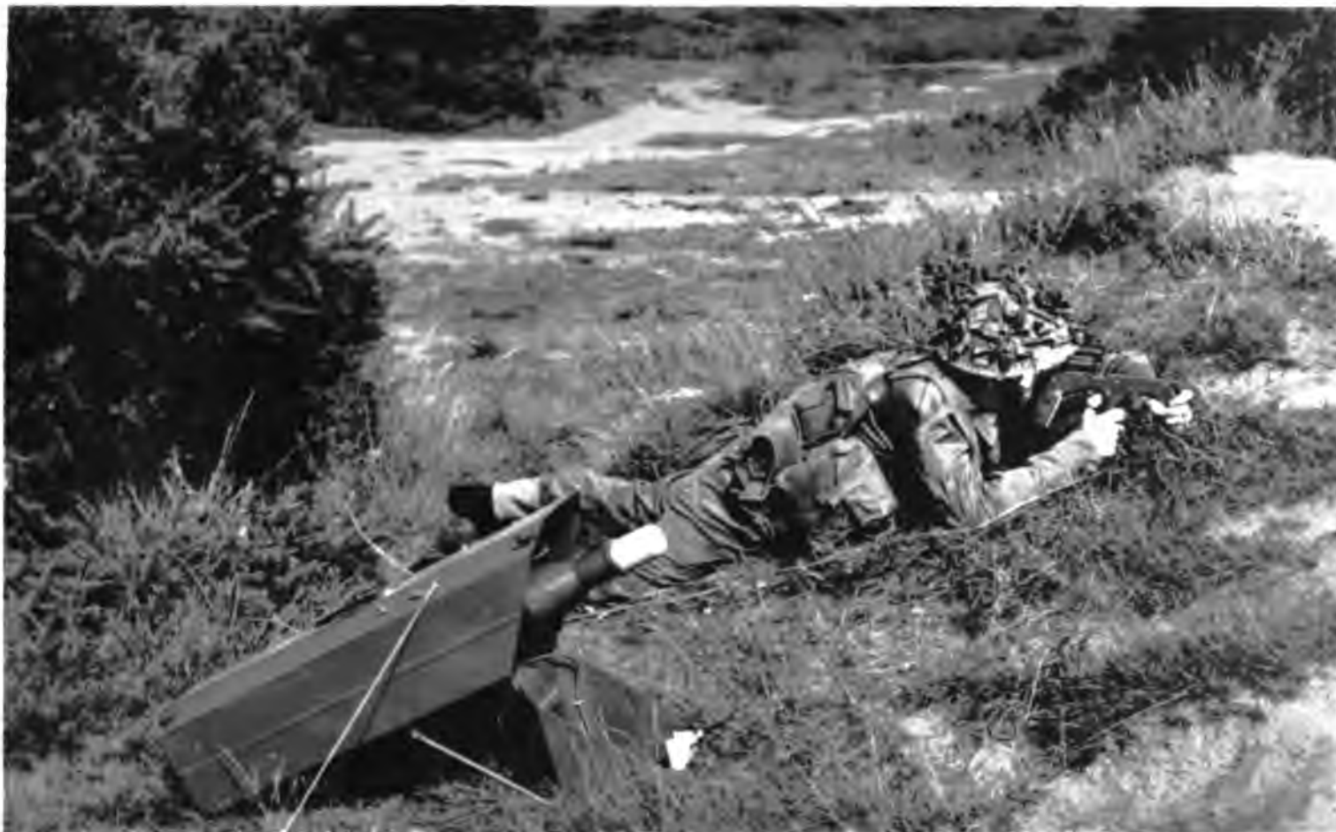
The Vickers Vigilant man-portable anti-tank missile which is now in production for official trials by the British Army. The Vigilant is claimed to be more accurate than any comparable weapon, and to be lethal to the heaviest known armour. An infantryman can use it after only five hours simulator training plus the firing of three or four rounds
