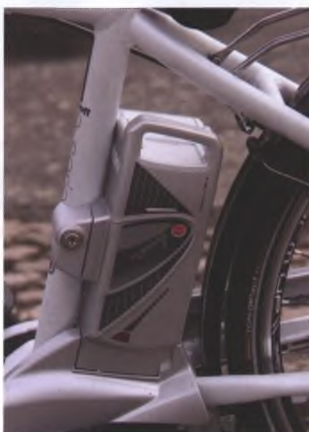
The battery locks into place and is removed with a key.
